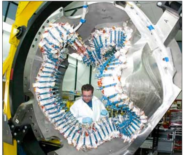
Winding of an NCSX modular field coil.
