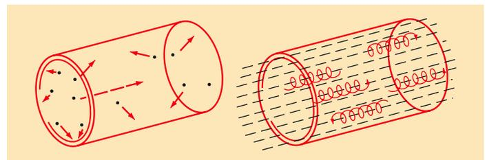
At left: Motion of charged particles without magnetic field, and at right with magnetic field.
