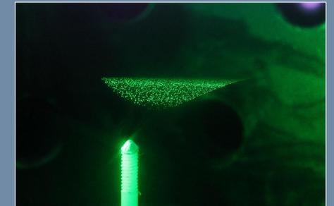
Figure 7. A dust cloud (about 1" wide) forms directly above the POM support (see Fig. 1).
