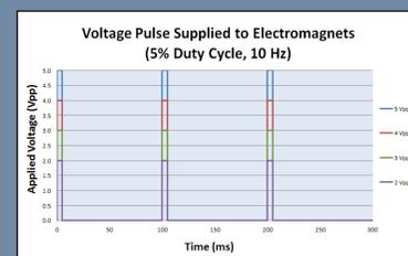
Figure 3. Voltage waveform supplied to the electromagnets. Different voltage amplitudes are used to vary the drop rate.
