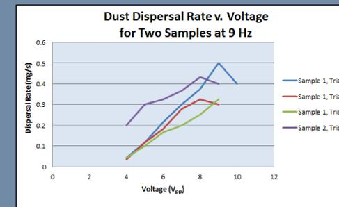
Figure 5. Dust dispersal rates for two dust samples.
