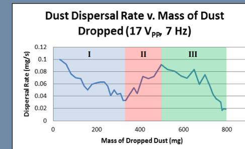
Figure 6. Stage I: Dust compacts around agitator. Stage II: Agitator creates an open space on the mesh. Stage III: Rate decreases as total dust dropped increases.
