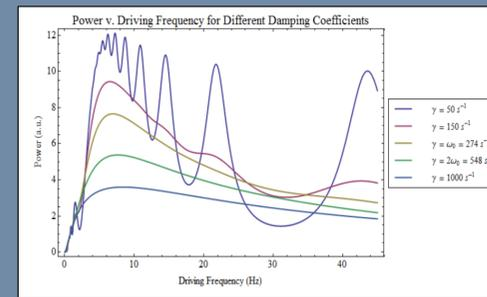
Figure 4. Power absorbed by the shaker for several damping coefficients.
