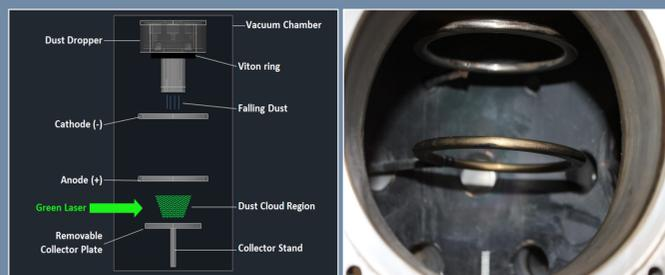
Figure 1. Left: Diagram of the DPX setup. Right: Photo of the cathode (top), anode (middle), and POM support (bottom) in the vacuum chamber.
