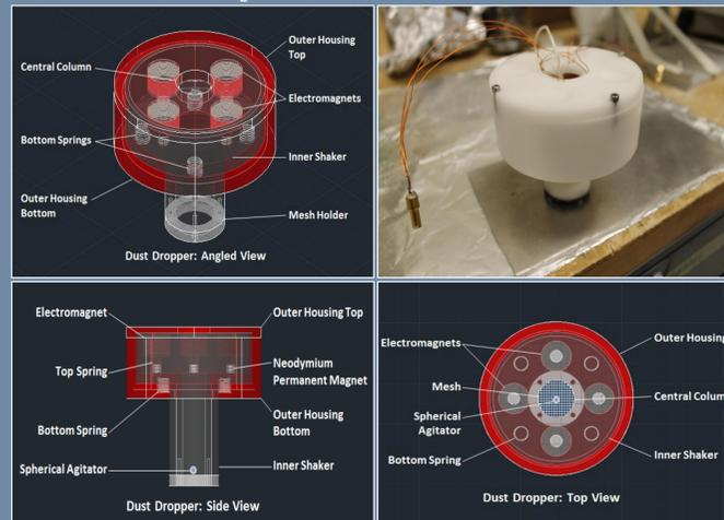
Figure 2. Diagrams of the dust dropper from three views. Upper Right: Photo of the dust dropper.
