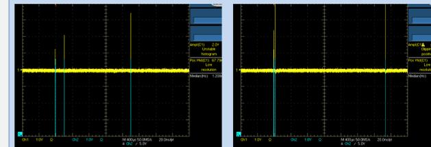
Some isolated voltage spikes in the range of 1-4 V mimic behavior observed for carbon.
