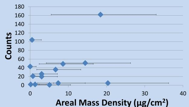
Trials used "PF-5F" stainless steel particles<sup>9</sup> dropped through a triple mesh. The power supply current limit was 2 mA and the SCA lower threshold was 0.4V. No clear correlation of counts with mass density was apparent. Approximated sensitivity: 4 counts/μg/cm<sup>2</sup>
