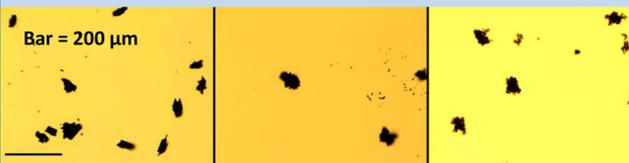
Count Median Diameter: 5.87 μm      Count Median Diameter: 4.78 μm      Count Median Diameter: 37.30 μm
