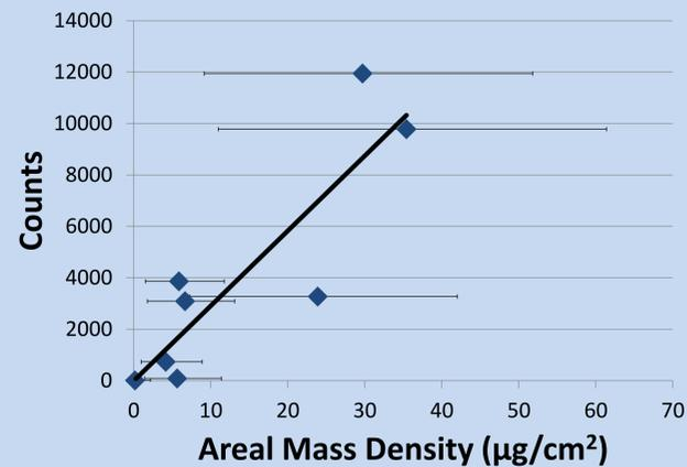
Carbon sensitivity, determined from a linear fit including the origin, is 291 counts/μg/cm<sup>2</sup>, a result that compares well to a previous result of 239 counts/μg/cm<sup>2</sup><sup>5</sup>
