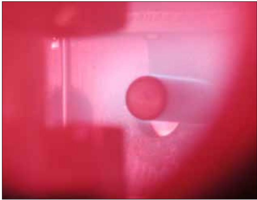
**View of the interior of LTX during the plasma glow procedure which deposited lithium coatings on the liner. The bright red-colored glow is characteristic of lithium.**
